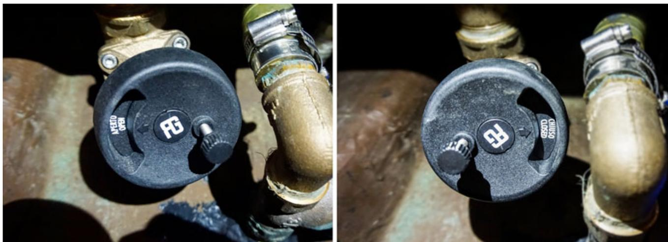
Furthermore, thanks to their efficient functioning, **we will never be obliged to force the group ” valve – water intake – hull” and this is another very important aspect.** Traditional valves are equipped with levers and, when the latter are blocked, the force we use to unblock them significantly affect the group we have just mentioned, **with the risk of compromising both sealing ( waterways) and resistance of each parts ( sea water intakes and valve levers).**
