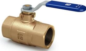
This full bore ball valve by Guidi features a body and a body end made of CC499K bronze as well as a ball in PPS, a semi-crystalline thermoplastic with excellent mechanical and chemical resistance properties that are retained at high temperatures. This valve, currently under production, is subject to a special surface treatment of the ball, to improve its encrustation-resistant properties.
